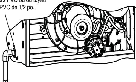
DRAINAGE PAR LA GAUCHE ACHÉMINÉ DERRIÈRE L'ÉVACUATEUR
